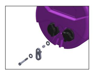
Install lockout plate with original bushing, washers and (1) - M6 x 60 screw to the K-MASS Electronics Cover. Apply blue Loctite thread locker (included) to this bolt only (important).
