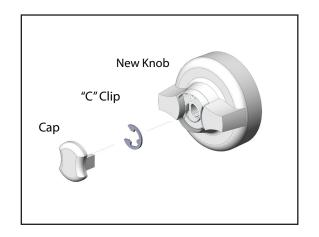
Remove center caps from existing plastic knobs. Remove "C" clips and actuator knobs and retain for re-installation. Remove knob shafts and plastic washers.
