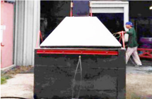
Thermal Designs medium size (4' x 4' x 3') fire test chamber
