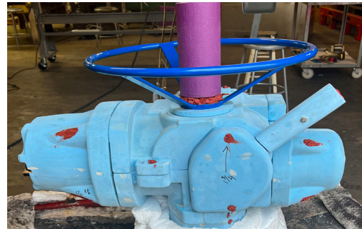
Actuator before fire test. Mounted on the base of the oven before sides and top of the oven are installed
