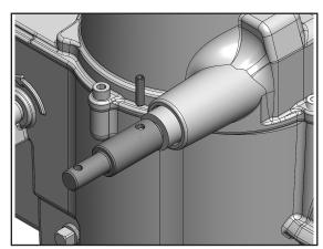
**Step 2** Install Handwheel Shaft Extension (included FRIQ1S-1401) using Roll Pin (FRIQ1S-1402 included).
