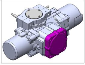
Install the Terminal Cover (FRIQ1S-1703) and loosely bolt to the Gearcase Covers with (4) - M8 x 30 socket head cap screws.
