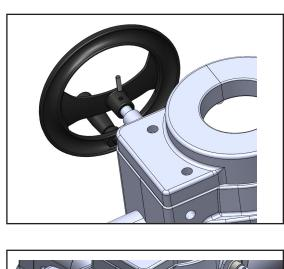
**Step 16** Install the handwheel on the Handwheel Shaft Extension using the split pin provided.
