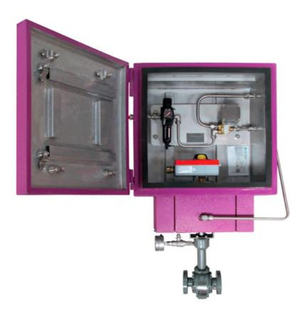
K-CABS are custom designed and fabricated **K-MASS** coated EN 1.4301 (304) grade stainless steel, instrument and electrical component cabinets. K-CABS are tested to provide a minimum of 30 minutes of protection in a 1093° C/ 2000° F hydrocarbon fire. (UL1709 fire test curve as per API 2218)
