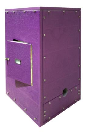
**K-MASS** LITE enclosures are field installable, stainless steel enclosures manufactured by molding an expanded, open cell foam version of **K-MASS** into a 304 stainless steele frame. **K-MASS** LITE fireproof enclosures have been fire tested to UL1709 fire test curve for 60 minutes.
