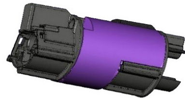
Knob extension showing machined K-MASS extension and new knob
