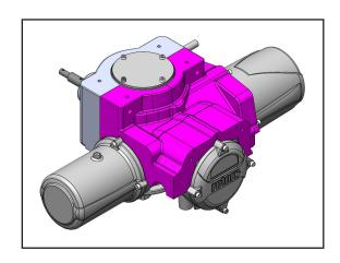
Attach the terminal side of the Top Gearcase Cover (FRIQ2S-2101) next to motor with (2) - M8 x 40 socket head cap screws.
