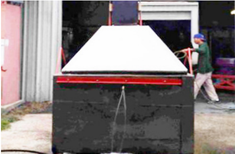
Thermal Designs medium size (4' x 4' x 3') fire test chamber
