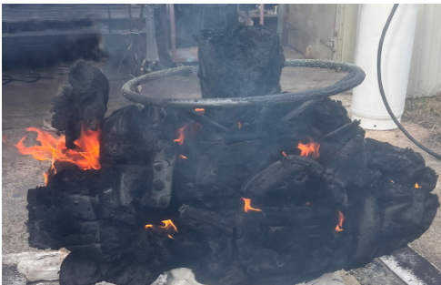
Actuator after the test showing the black, expanded K-MASS char
