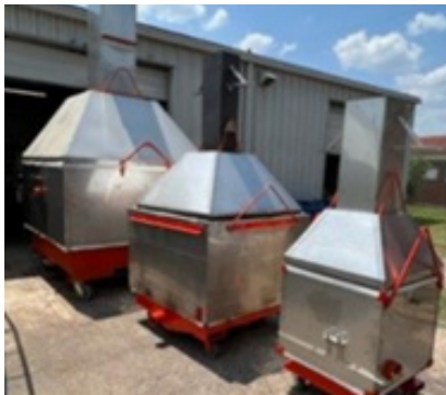
Our three fire test chambers 6'x6'x4' 4'x4'x3' 2'x2'x2'
